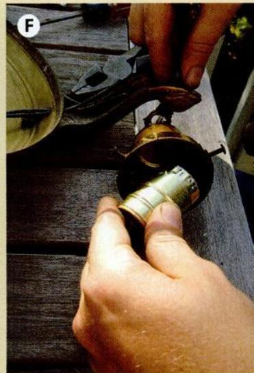
**A breakdown of socket parts (D)—body, insulating sleeve, outer shell and cap—old (left) and new (right). Estimate how much wire you'll need to run through the arm (leave extra), then strip the neutral wire, bend the end, twist it behind the silver screw, and tighten (E); repeat with the hot wire on the brass screw. Return the base to its lining and shell, place the cap inside the socket housing, then snap the socket into the cap (F).**
