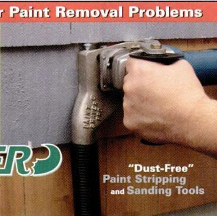
The **PaintShaver® Pro** will strip 1 square foot of lead or regular paint from clapboards, shingles, or any flat surface **in 20 seconds** while collecting the debris into any vacuum.
