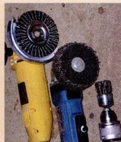
Stripping tools include stainless steel and brass brushes and angle grinders and drills with knotted wire wheels, brushes, or non-metallic mesh discs.
