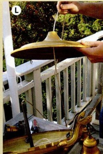
**wired, gather all of the neutral socket wires, including the one threaded through the main arm (J) and twist them together, then cap with a wire connector (K). Repeat the process with the remaining hot wires. Your fixture is now ready to be reassembled (L) and hung back in place.**
